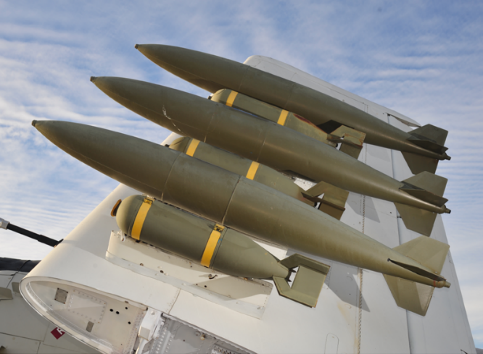
Ordnance fills the bottom of the folded wing of an A-1 Skyraider attack aircraft. Chris Hunkeler
